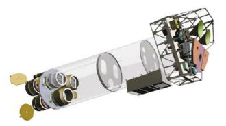
Fig. 1. "Open" view of the XMM-Newton observatory. To the left the three mirror modules (with the RGA units mounted behind two of them) can be seen, while at the right the backend of the instrument platform with all the radiators is visible
