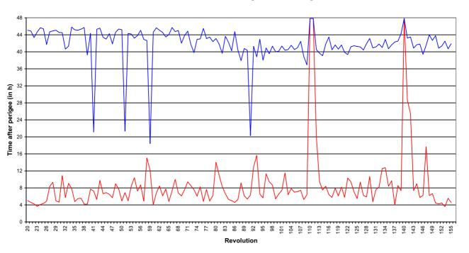
Fig. 4. Time throughout the 48 hour XMM-Newton orbit that the radiation levels are not exceeding critical limits. The red line traces the time after perigee, at which safe operations can begin. The blue line displays the equivalent period *before* perigee. The two large solar flares in summer 2000 can be clearly identified
